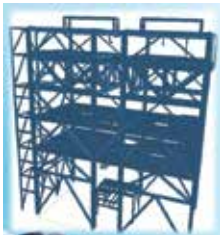
3D-Staad Model of Process structure
